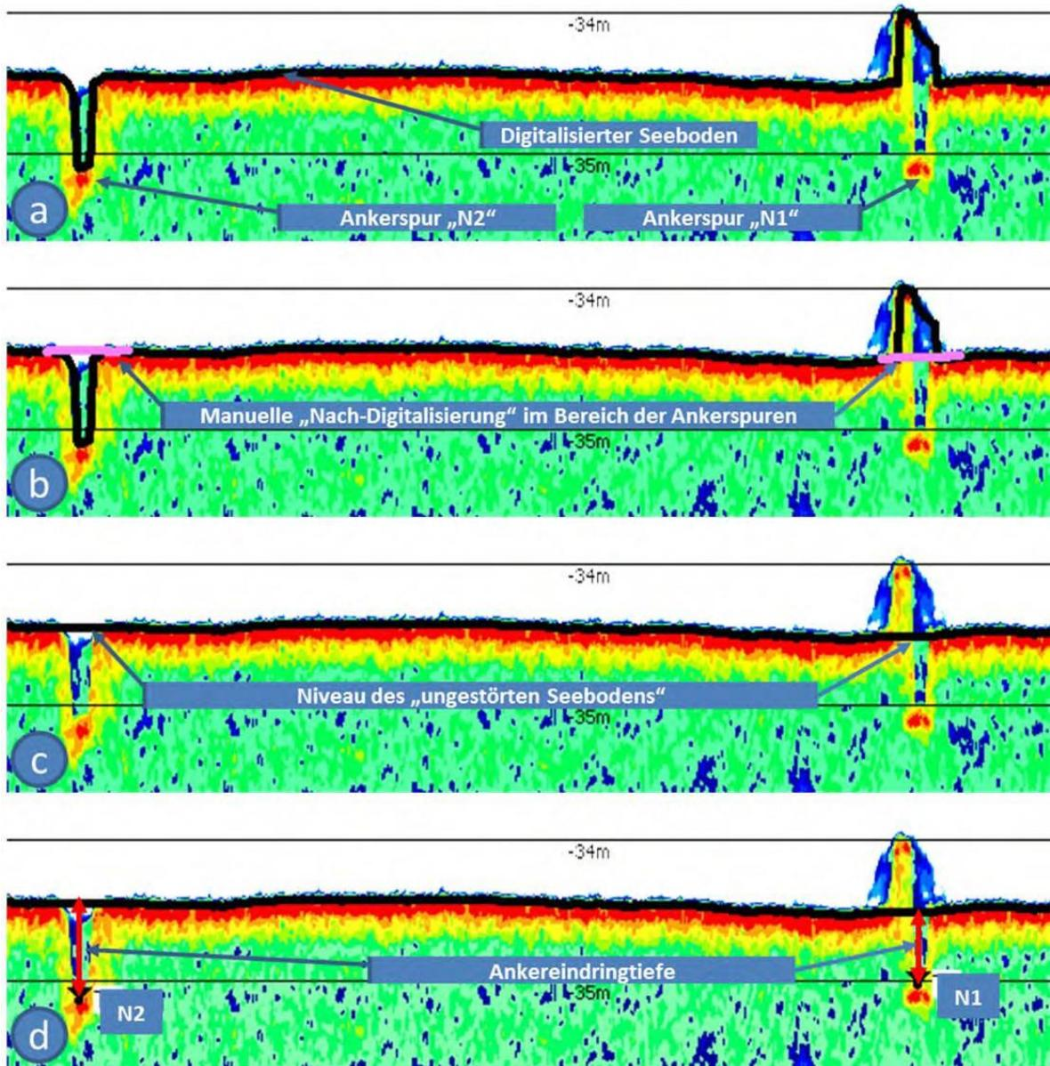
**Plate 11: Obtaining the anchor penetration depth from SES profiles**
