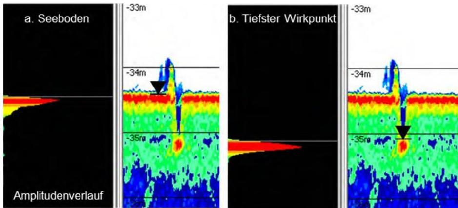
**Plate 12: Digitisation of SES signal amplitudes**
