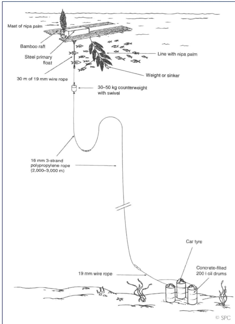
**Figure 1:** Schematic illustration of a FAD (<http://www.fao.org/3/i3087e/i3087e.pdf>)
