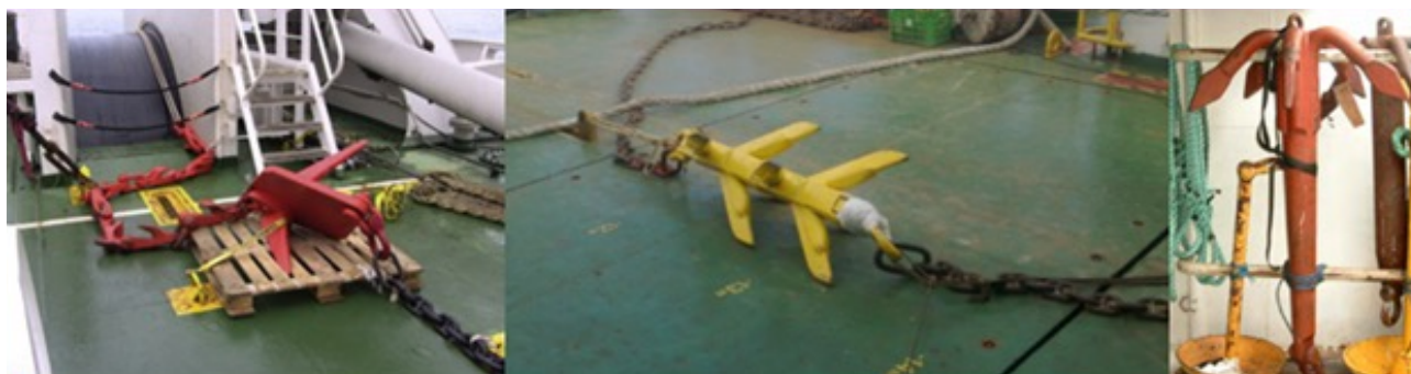
Figure 6. A grapnel array used to clear the seabed of debris and out of service cables. Source: courtesy of ICPC
